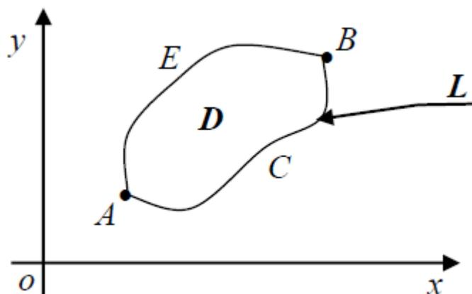
$$\oint_L Pdx + Qdy = \iint_D \left( \frac{dQ}{dx} - \frac{dP}{dy} \right) dx dy$$
